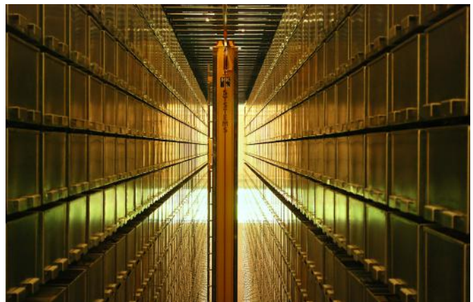
Automated Storage and Retrieval System at the UBC Library. Photo courtesy of UBC Library Communications.
